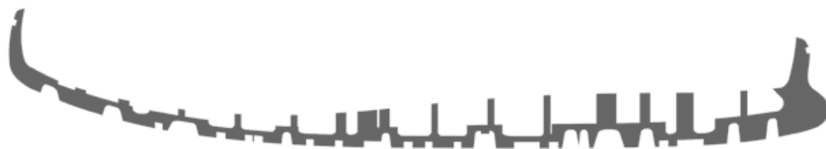
Outsole cross-section | Cleatdepth 4.0 – 3.0 mm | Effective thickness 1.5 mm
