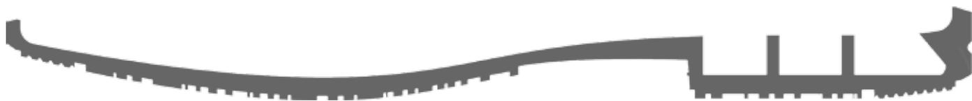
Outsole cross-section | Cleatdepth 2,7 mm | Effective thickness 4,0 mm
